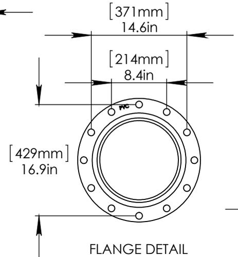
STAINLESS STEEL (316) 5/8" (16mm) THREADED ROD, WASHER, LOCK WASHER, & NUT. THREADED ROD LENGTH 9" (230mm) WITH 6" (150mm) EMBEDMENT. USE MINIMUM 6 ANCHORS.
