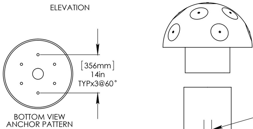
1/2" (13mm) STAINLESS STEEL (316) THREADED ROD, WASHER, LOCK WASHER, & NUT. SUGGESTED 7" (180mm) THREADED ROD WITH 6" (150mm) EMBEDMENT.
