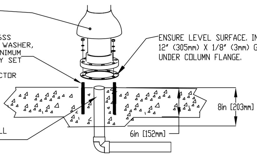
WATERFEED 2" (50mm) PVC SCH 40 PIPE CUT CLOSE PRIOR TO INSTALL TO ALLOW FULL DRAINAGE (WINTERIZATION)
